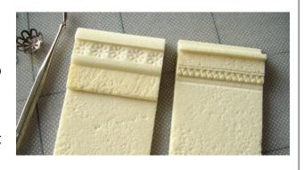
The thick (10mm) version of Kapa-line foam can also be ideal for building up whole structures, especially if all paper is removed.
