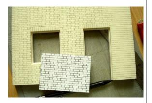
I recommend taking the trouble to draw up a small sample of scale brickwork which can then be used to mark spacings.
