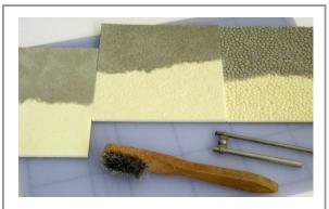
As well as using pencil or wire brush to create effects, I often impress the ends of metal tubes, in this case creating the effect of street cobbles.
