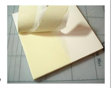
The foam is polyurethane (different from the polystyrene in standard foamboard) and is stronger, much denser though still soft.
